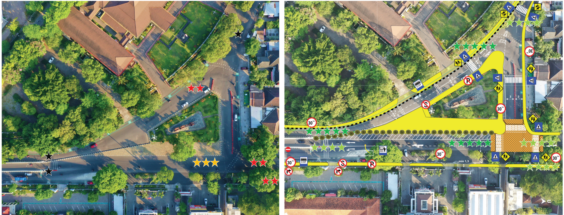
Figure 4. Manahan flyover area: before (left) and proposed design after the intervention of star rating (right)
