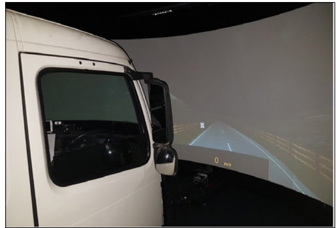
Figure 1. Truck simulator exterior with forward road scene projection
